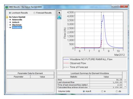
This is a significant hydrograph just from the rain that has already fallen, but if we zoom in we see that the computed flows are higher than the observed, meaning that the soil is dryer than what the model is set to.
