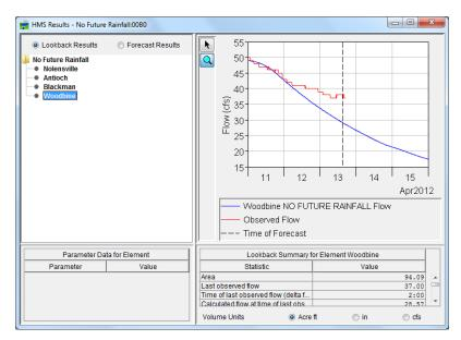
This is relatively good, considering this is an event oriented model. We could modify the ground water component in the model to contain another sub-layer so that the curves match, but it wouldn't have much impact during high flows. If we wanted to keep our calibration for the next forecast, we'd "Save HMS to base", generally a good idea.
