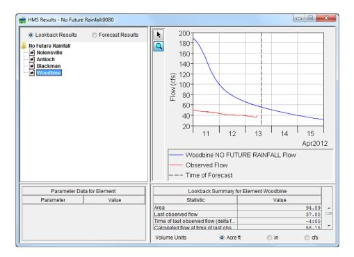
For this time frame, there was no significant precipitation and little to calibrate to. The base flow is significantly off. We can, and will, adjust it, but we cannot determine a good estimate of soil moisture from the plot; for that we'll need experience. However, the plot shows that we're not in an event, so the results for this time are probably not as important. If we had a rising hydrograph, we could do a much better job of estimating soil moisture parameters.
