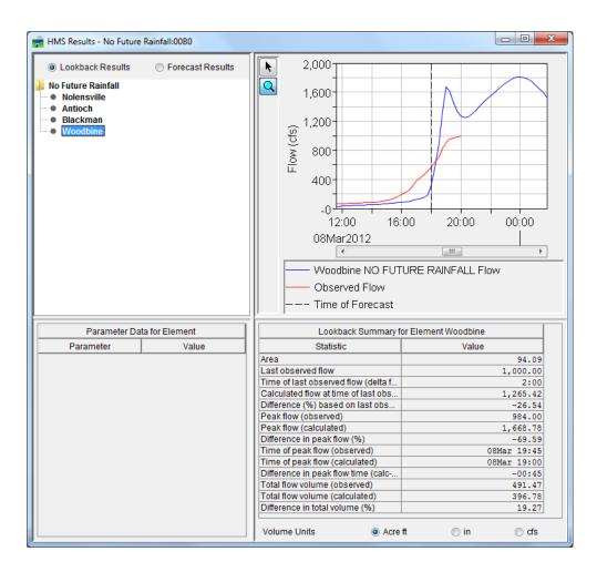
We can continue to adjust the loss rates to bring the computed curve closer together. The information in the bottom of the table provides some comparison information. In the above plot, we would only have flow up to 1800, the time of forecast. At that time, it looks like were actually have our loss rates set too high.
